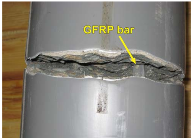
Pipe Rupture on Tension Surface – Faster Load Rate
