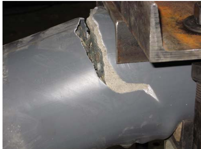
Pipe Rupture and Bulging – Faster Load Rate
