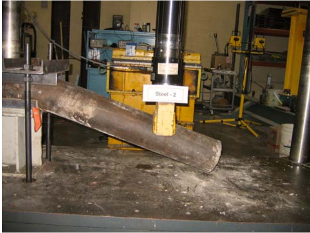
Failure Condition – Slow Load Rate
