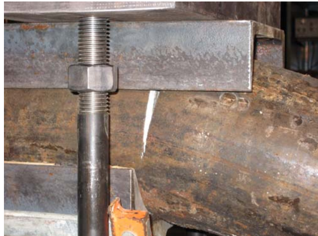
Pipe Rupture and Bulging – Faster Load Rate
