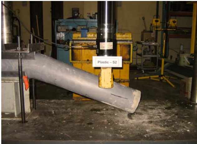
Failure Condition – Slow Load Rate
