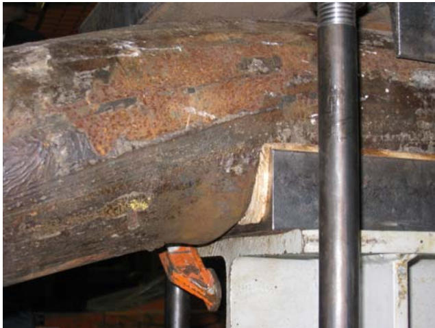
Distortion and Bulging of Pipe – Slow Load Rate
