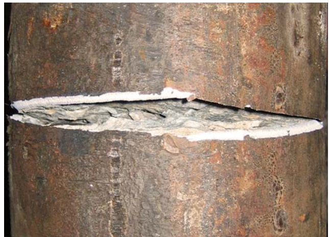
Pipe Rupture on Tension Surface – Faster Load Rate
